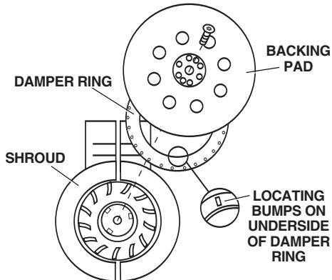
of locating groove. Loosen the two screws on shroud just enough so you can separate shroud approximately 1/4 inch. Align locating bumps on damper ring with cut outs in shroud and depress ring with thumbs until shroud seats into groove completely around ring, then tighten screws.
